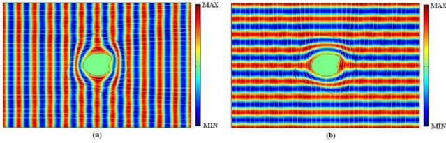
FIG. 2. (Color online) The contour plots of the electric fields  $E_z$  of the TE wave incident from (a) left and (b) bottom sides on an irregular shaped cloak without singularity. (The white lines indicate directions of the power flow).
