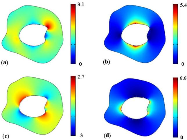
FIG. 3. (Color online) The contour plots of the material parameters (a)  $\varepsilon_z$ , (b)  $\mu_{xx}$ , (c)  $\mu_{xy}$ , and (d)  $\mu_{yy}$  of the irregular cloak by setting  $C_0 = 5$  in Eq. (8).
