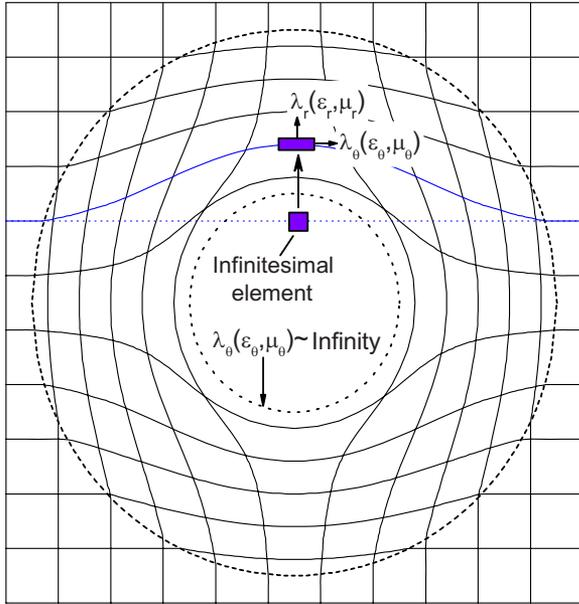
FIG. 1. (Color online) The sketch for the formation of singularity in material parameters of a cylindrical cloak.
