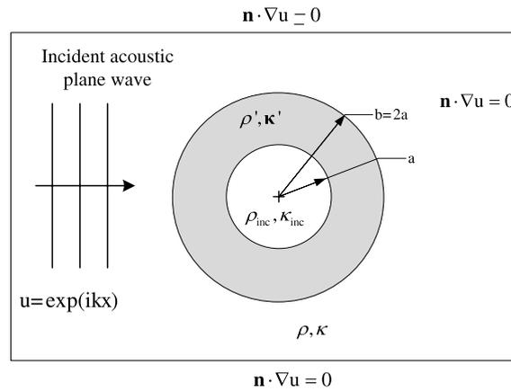
Fig. 3. Computational domain and simulation for a left-incident acoustic cloak based on Helmholtz equation.
