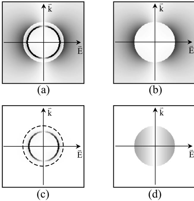
FIG. 5. Contour plots of the distribution of radial component of the scattered electric field in the  $E$  plane for a doubly coated sphere (left) and its effective sphere (right) [ $\epsilon_1=-5$ ,  $\epsilon_2=3$ ,  $\epsilon_3=10$ ,  $\mu_1=\mu_2=\mu_3=1$ ,  $r_1=\lambda_0/100$ ,  $r_2=1.1r_1$ , and (a,b)  $r_3=1.2r_2$ ; (c,d)  $r_3=1.31r_2$ ].
