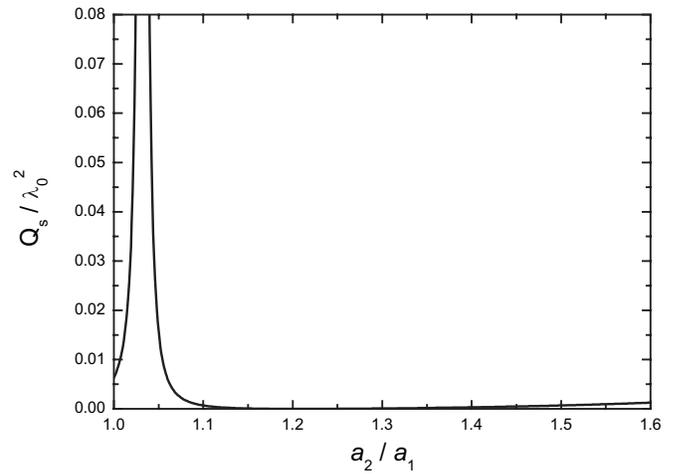
FIG. 9. Normalized total scattering cross section of a coated sphere as a function of ratio  $a_2/a_1$  for a fixed inner core ( $\epsilon_1=-3$ ,  $\epsilon_2=10$ ,  $\mu_1=\mu_2=1$ , and  $a_1=\lambda_0/20$ ).
