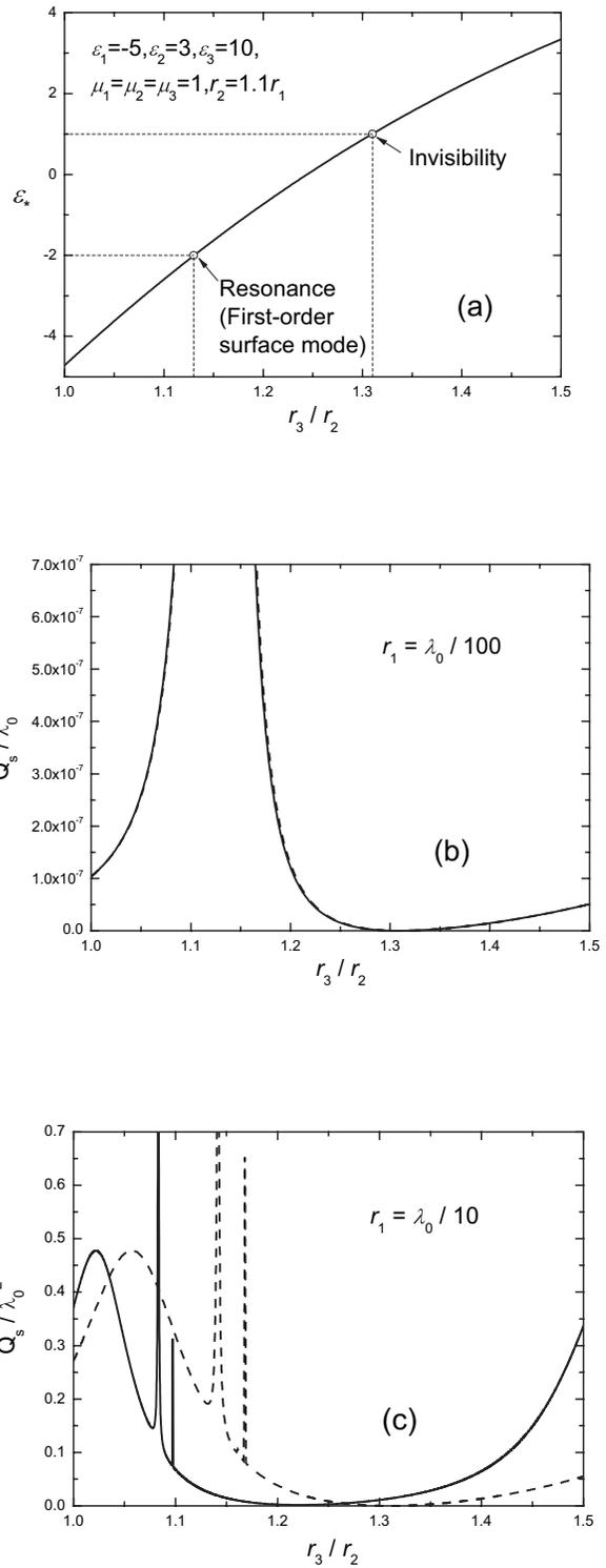
FIG. 4. (a) The effective permittivity  $\epsilon_*$  of a doubly coated sphere assemblage calculated from Eq. (4) and (b,c) normalized scattering cross section of a doubly coated sphere (the solid line) and effective homogeneous sphere (the dashed line) with the permittivity  $\epsilon_*$  and radius  $r_3$ , vs the ratio  $r_3/r_2$  for different  $r_1$ .
