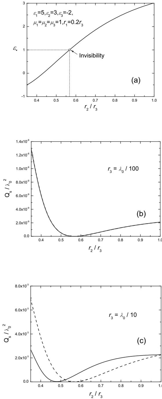
FIG. 3. (a) The effective permittivity  $\epsilon_*$  of a doubly coated sphere assemblage calculated from Eq. (4), and (b,c) normalized scattering cross section of a doubly coated sphere (the solid line) and effective homogeneous sphere (the dashed line) with the permittivity  $\epsilon_*$  and radius  $r_3$ , vs the ratio  $r_2/r_3$  for different  $r_3$ .
