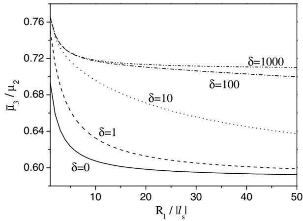
Fig. 2. Effective shear modulus as function of void radius for the surface of type I for different values  $\delta$ .
