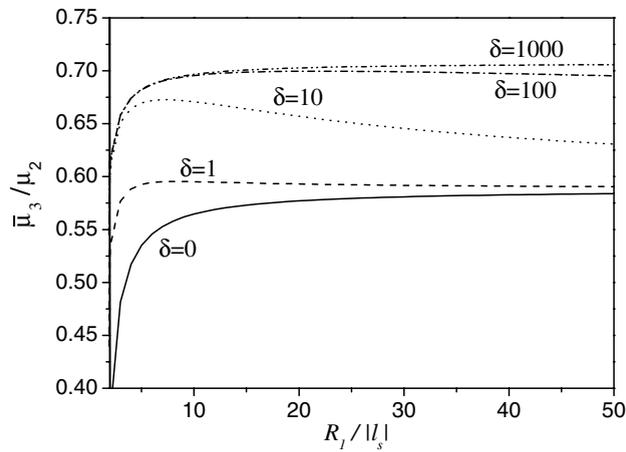
Fig. 3. Effective shear modulus as function of void radius for the surface of type II for different values  $\delta$ .
