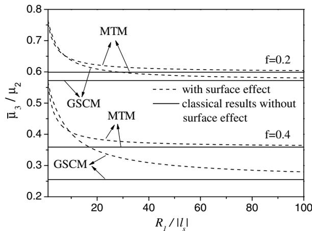
Fig. 5. The shear modulus of composite with the surface of type I predicted by MTM and GSCM ( $\delta = 1$ ) for two different void volume fractions.
