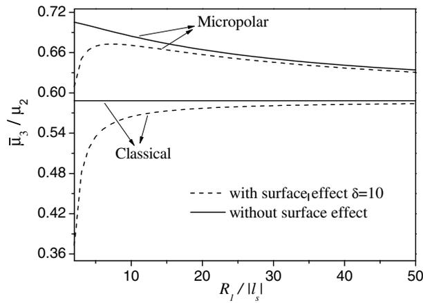
Fig. 4. Variation of the effective shear modulus as function of void radius predicted by different models with or without surface effect ( $\delta = 10$ ), for the surface of the type II.
