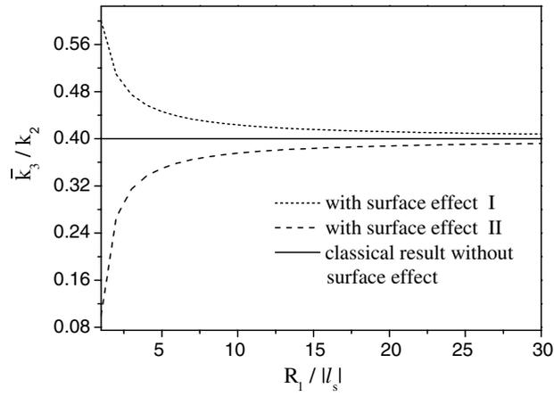
Fig. 1. Variation of effective modulus as function of void radius for two types of surface properties.
