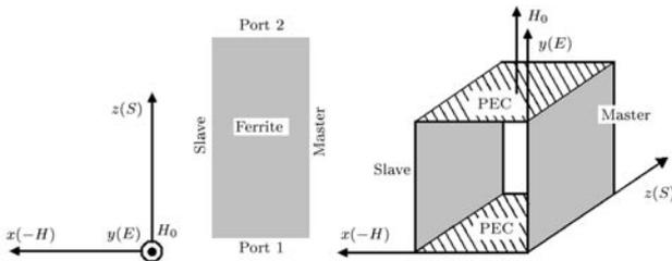
**Fig. 4.** Finite element model for a plate waveguide, periodic condition along the  $x$  direction. Top and bottom surfaces in the  $y$  direction are PEC, front and back surfaces in the  $z$  direction are two waveports.
