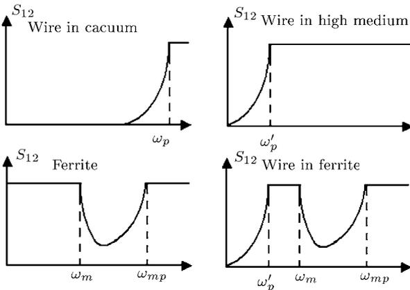
**Fig. 2.** Transmission property of WIRE, ferrite and their composite. Here  $\omega_m = \gamma \sqrt{H_0(H_0 + M_s)}$  is the ferromagnetic resonance frequency, and  $\omega_{mp} = \gamma(H_0 + M_s)$  is the anti-resonance frequency.
