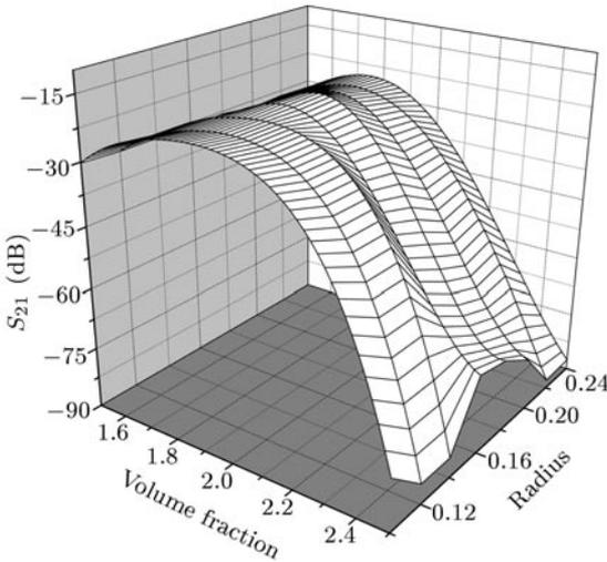
Fig. 8. Influence of ferrite volume fraction and WIRE radius on transmission property  $S_{21}$ .
