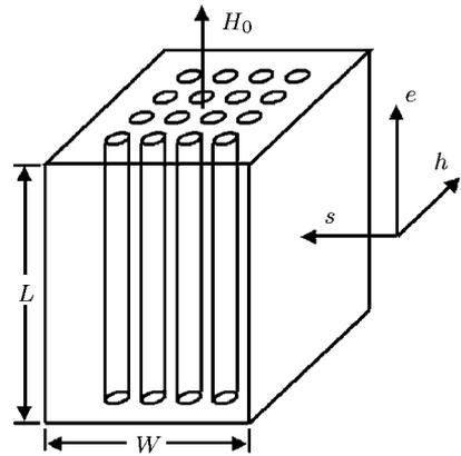
Fig. 1. WIRE structure in ferrite matrix proposed by Dewar.<sup>[13]</sup> The TEM wave is incident along the  $s$  direction, electrical field and static magnetic field are parallel to the WIRE.
