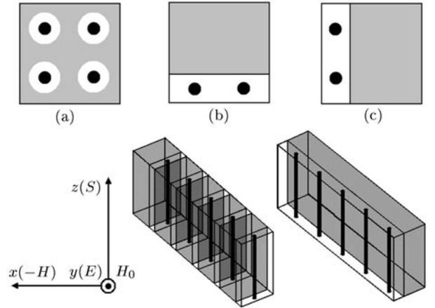
**Fig. 3.** Top view of models to reduce electromagnetic coupling. The TEM wave is incident along the  $z$  direction, with magnetic field parallel to  $x$ , the electric field and applied static magnetic field parallel to  $y$ .
