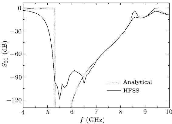
**Fig. 5.** Comparison between analytical results (dotted line) and HFSS result (solid line) for transmission property  $S_{21}$ .
