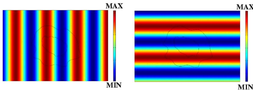
Fig. 4. Simulation of the acoustic wave without any obstacle. Left: left incident. Right: bottom incident.
