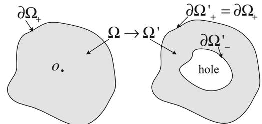
Fig. 1. Transformation from the region  $\Omega$  to  $\Omega'$  for constructing a perfect cloak. The outer boundary  $\partial\Omega_+$  of the region  $\Omega$  is kept unchanged, and the point  $\mathbf{O}$  inside of  $\Omega$  is transformed to the inner boundary  $\partial\Omega'_-$  of  $\Omega'$ . Except a point  $\mathbf{O}$  and  $\partial\Omega'_-$ , the transformation is everywhere one-to-one and differentiable.
