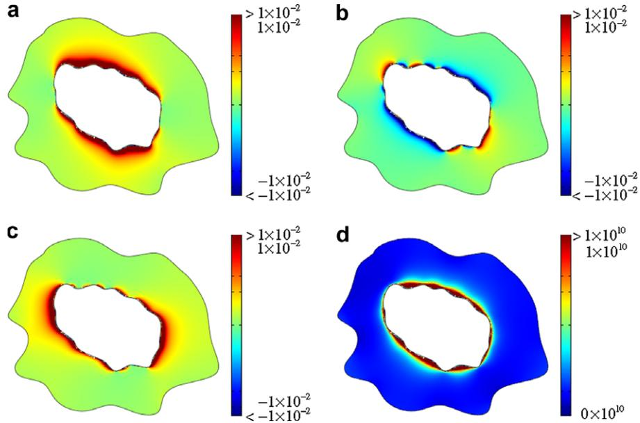
Fig. 7. Values of the non-vanishing components of the mass density tensors of the designed cloak, (a)  $1/\rho'_{xx}$ , (b)  $1/\rho'_{yy}$ , (c)  $1/\rho'_{yy}$ , and (d) bulk modulus  $\kappa'$ .
