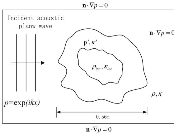
Fig. 2. Computational domain and simulation for a left-incident acoustic cloak based on Helmholtz equation.
