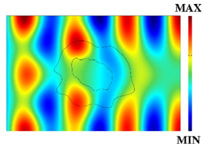
Fig. 5. Simulation of a left incident acoustic wave without the cloak layer.
