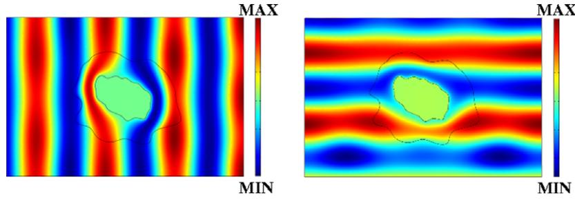
Fig. 6. Simulation of the acoustic wave with the designed cloak layer. Left: left incident. Right: bottom incident.
